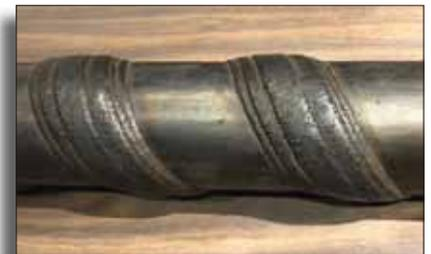
Crack-Free Hardfacing alloy with martensitic tool steel structure
