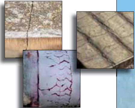
Chromium Carbide Hardfacing with stress relief cracks
