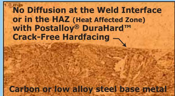
Postalloy® DuraHard™ Crack-Free hardfacing compatible with base metal chemistry will NOT lead to diffusion and spalling.
