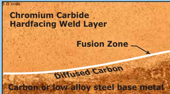
Hardfacing with chromium carbide results in an enriched **hard and brittle layer known as diffused carbon**, where the base metal meets the weld metal (white area in the photo above) leading to spalling and chipping.
