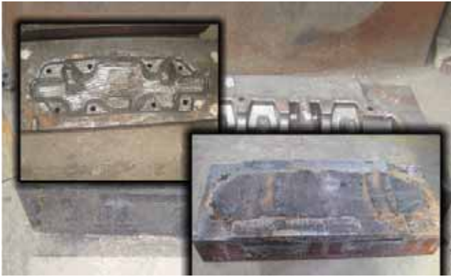
Crankshaft forging die showing gouged and repaired weld with Postalloy 2235 buildup and 2755 hardfacing material
