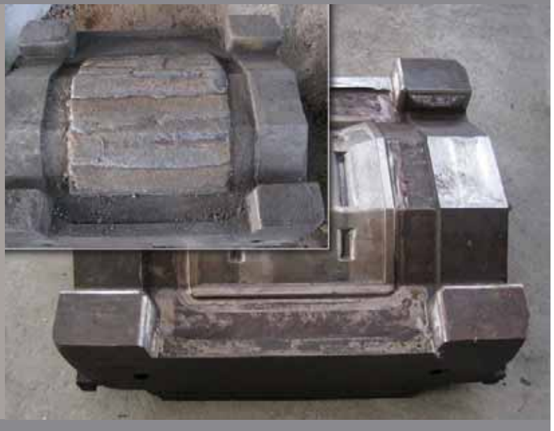
Forging die weld-repaired with Postalloy 2235 as a buildup material and 2747 as a hardfacing material
