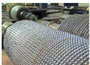
Hardfacing can be used on cane rolls to create a hook profile to increase productivity as well as increasing service life up to 300% or more.
