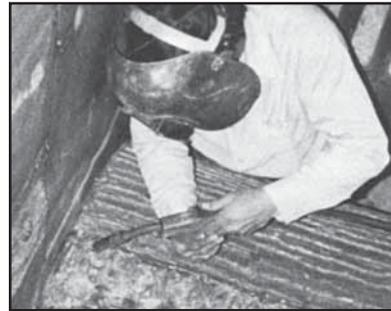
Crusher Roll hardfaced with 2820-SPL after application of Postalloy 2865-FCO
