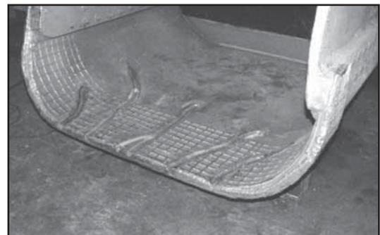
Bucket prepped for repair welding with 3044-FCG.
