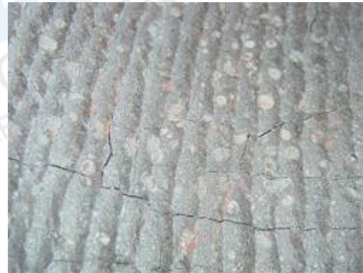
Stress Cracks in Chromium Carbide.
