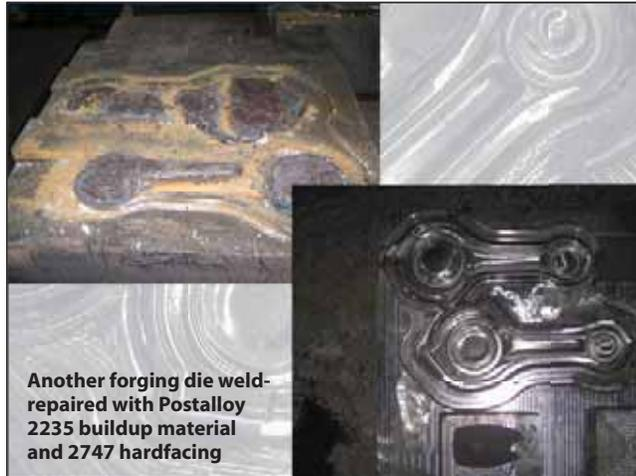
**Another forging die weld-repaired with Postalloy 2235 buildup material and 2747 hardfacing**
